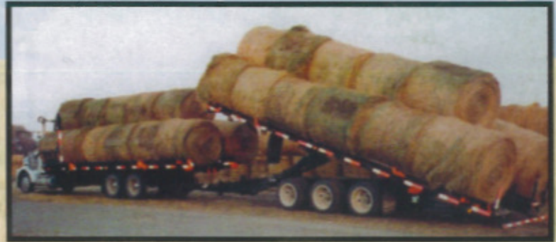
Unload truck & trailer deck without jackknifing
